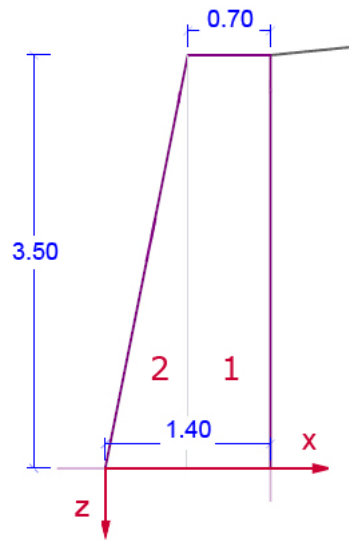
Figure 5: Dimensioning of cross-section
